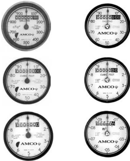
with an "L" shaped gasket, then roll sealed. To assure easy reading, the totalizer wheels are large and color coded. The applicable size, model, registration, part number and date code are printed on the calibrated dial face. Moving clockwise during operation, extra thin sweep hands do not interfere with meter reading, and the low-flow indicator will detect plumbing leaks.
