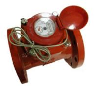
Magnetic Drive The magnetic drive design eliminates all miscouplings associated with conventional right angle drives. Excess torque is eliminated in the encased undergear assembly, ensuring constant magnet coupling.
